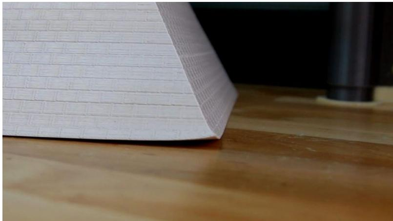
Example of Warped Part Without Proper Adhesion
